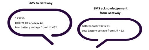
In this example a Low battery voltage indication will generate the following:
